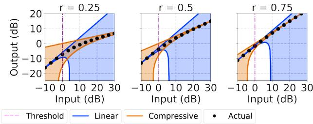
Fig. 6. Static compression characteristic of dynamic range compressions  $\mathbf{G} \mapsto (\mathbf{G} + \delta)^r - \delta^r$ , as a function of the ratio  $\frac{\mathbf{G}}{\delta}$  between input magnitude  $\mathbf{G}$  and soft threshold  $\delta$ , for different values of  $r$ : 0.25 (left), 0.5 (middle), and 0.75 (right). Solid lines and shaded areas respectively denote asymptotic bounds and their corresponding error margins, as proved in Proposition III.4.
