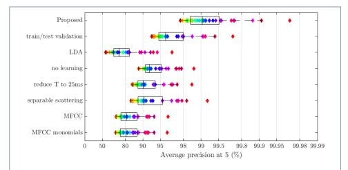
**Figure 6** Impact of different processing architecture or protocol designs. For each condition, the central mark indicates the median, and the bottom and top edges of the box indicate the 25th and 75th percentiles, respectively. The performance achieved for each reference clustering is depicted by a lozenge whose color is chosen arbitrarily but consistently across conditions. See discussion section for details.
